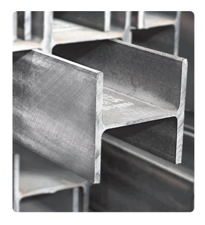
H-Beam is another product coming out from our hot rolled mill. It is the structural steel profile shaped like an H in section. The horizontal elements of the "I" are flanges, while the vertical element is the web. The web resists shear forces while the flanges resist most of the bending moment experienced by the beam. Beam theory shows that the H-shaped sections is a very efficient form for carrying both bending and shear loads in the plane of the web.
