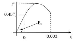
• Modulus of elasticity of concrete is automatically calculated and displayed by the program using f'<sub>c</sub>, w<sub>c</sub>, and the following relationship<sup>3</sup> of the code. User is given the option to override the code value and specify a user defined substitute.
